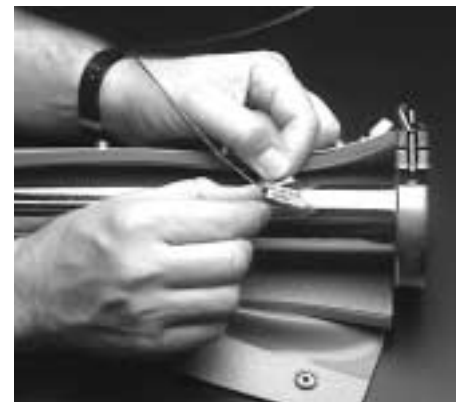
Self-adhesive Kapton thermocouple
